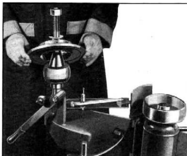
Fig. 9—Installing Leveling Plate
