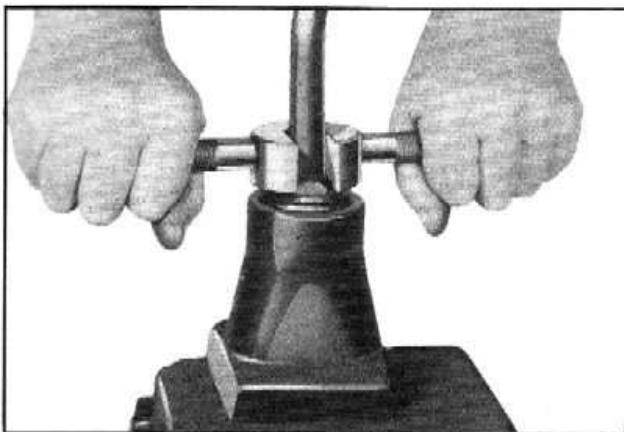
Fig. 18—Removing Gearshift Lever—Conventional Model
