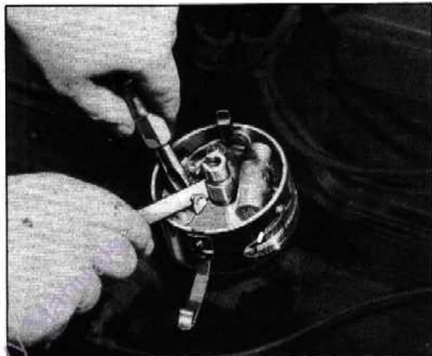
Fig. 40—Adjusting Distributor Breaker Points
