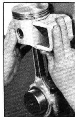
Fig. 31—Checking Piston and Connecting Rod Assembly
