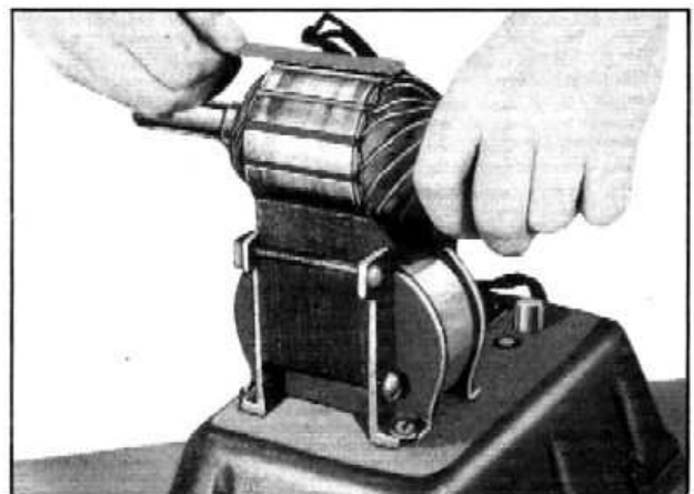
Fig. 11—Armature Test for Short
