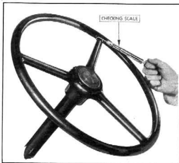
Fig. 3—Checking Worm Bearing Adjustment
