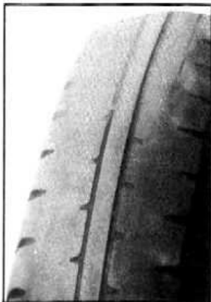
Fig. 3—Tire Wear Due to Under Inflation
