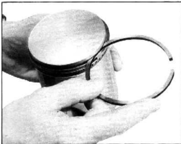
Fig. 6—Checking Ring Fit in Groove
