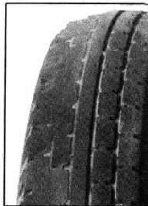
Fig. 2—Tire Wear Due to Improper Camber
