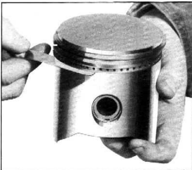
Fig. 7—Checking Piston Ring Clearance
