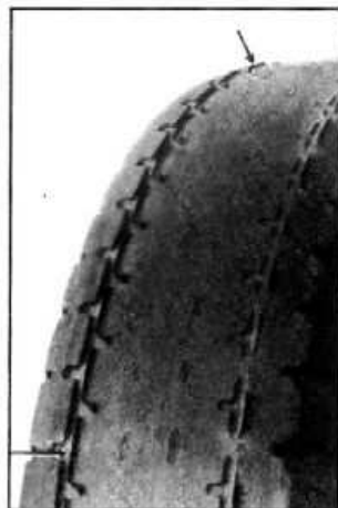
Fig. 4—Tire Wear Due to Improper Toe-In or Toe-Out
