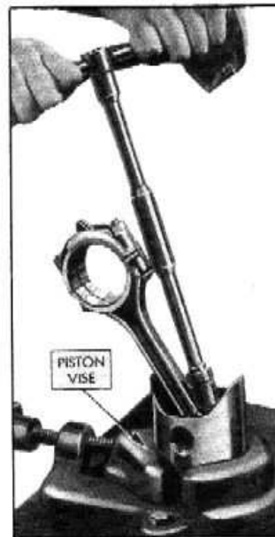
Fig. 30—Assembling Connecting Rod to Piston
