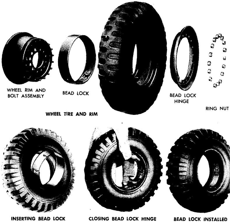
Figure 195—Bead Lock Tire and Rim Mounting and Dismounting
